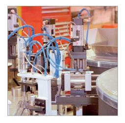
TPU Presto Tubing is a highly flexible tubing for demanding applications. It is easy to install due to its small bend radius and kink resistance.
