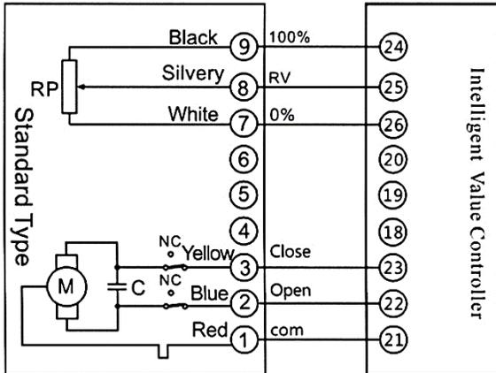
Picture 4 : wiring of the standart adjust type motor (setMd=1)
