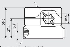
Gauge connection, integrated ø 9
